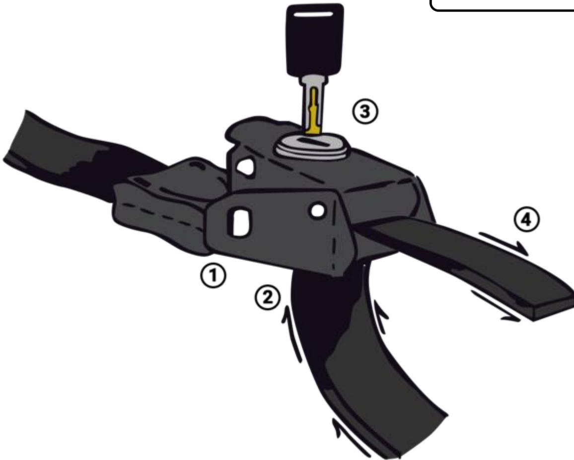
1. Push button and lift lever to open lock.
